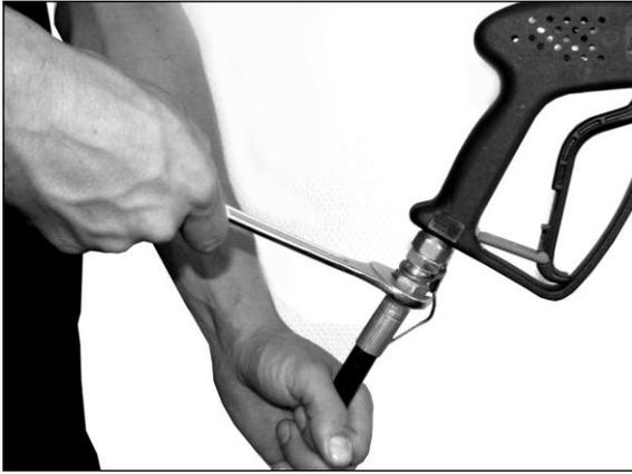
Now attach the coupling of the CO2 hose to the coupling of the CO2 Gun and secure this with an open-ended spanner.
