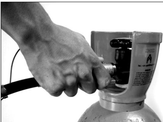
Unscrew the high pressure hose from the CO2 Gun and from the CO2 bottle.
