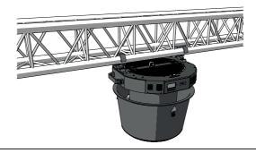
3 Make sure to use the safety steel to secure the machine to the truss. The safety steel can be attached to the safety eye on top of the machine.
