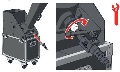
$\textbf{12} \quad \text{Connect the CO}_{\scriptscriptstyle 2} \text{ hose to the CO}_{\scriptscriptstyle 2} \text{ valve}.$
