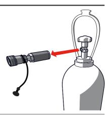
Connect a CO<sub>2</sub> Bottle to Hose Connector to a new CO<sub>2</sub> cylinder.
