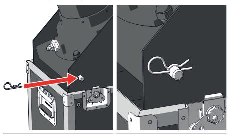
Set the angle of the woofer by aligning the back pinhole with one of the four predefined holes in the case.
