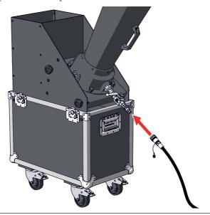
$\textbf{13} \quad \text{Make sure that the CO}_{\scriptscriptstyle 2} \text{ valve is in CLOSED position}.$
