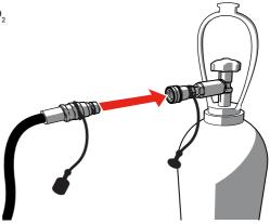
8 Move the manual CO<sub>2</sub> valve back in the CLOSED position.
