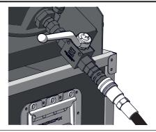
Close the connected CO<sub>2</sub> cylinder.
