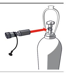
15 Connect the CO<sub>2</sub> hose to the CO<sub>2</sub> Bottle to Hose Connector on the CO<sub>2</sub> cylinder.
