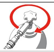
2 Move the manual CO<sub>2</sub> valve in OPEN position to release the pressure from the system.
