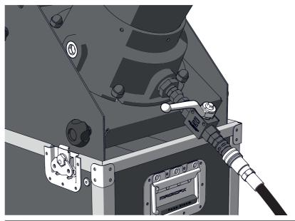
14 Connect the CO<sub>2</sub> Bottle to Hose Connector to a CO<sub>2</sub> cylinder.
