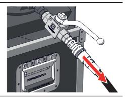
Disconnect the CO<sub>2</sub> hose from the CO<sub>2</sub> Bottle to Hose Connector on the CO<sub>2</sub> cylinder.
