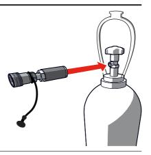
Connect the CO<sub>2</sub> hose to the CO<sub>2</sub> Bottle to Hose Connector on the new CO<sub>2</sub> cylinder.
