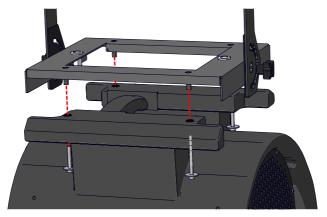
3 Mount the Doughty Quick-trigger Clamp (MFX3104) on top of the bracket with the supplied fasteners.
