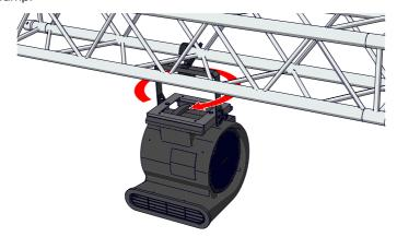
5 Rotate over the horizontal axis of the MAGICFX® FX-BLOWER by untighten and tighten the male star-nuts on both sides of the rotation bracket.
