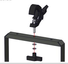
4 Hang the assembly below a truss and rotate over the vertical axis of the MAGICFX® FX-BLOWER by untighten and tighten de female T-nut underneath the clamp.
