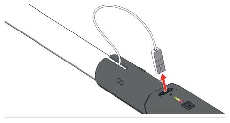
14 Remove the used cannon from the barrel and dispose it without harming the environment.
