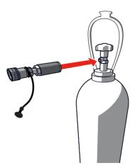
4 Connect the CO<sub>2</sub> hose to the CO<sub>2</sub> bottle to hose connector on the CO<sub>2</sub> cylinder.
