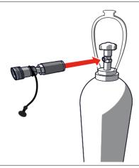
Connect the CO2 hose to the CO2 bottle-to-hose connector on the CO2 cylinder.
