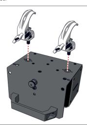
3. Mount the clamp firmly on a truss.
