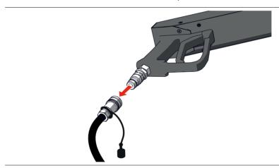
6. Disconnect the CO2 hose from the CO2 bottle-to-hose connector on the CO2 cylinder.
