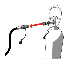
7. Remove the CO2 bottle-to-hose connector from the cylinder.
