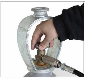
When the system is properly connected you can open the valves of the CO2 bottles. Check for leaks. When the gas hoses are not properly connected gas can escape. If this is the case then turn the couplings tighter until gas is no longer escaping.
