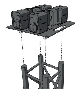
Secure the MAGICFX® BASEPLATE II correctly on a truss with conical pins and spring clips.
